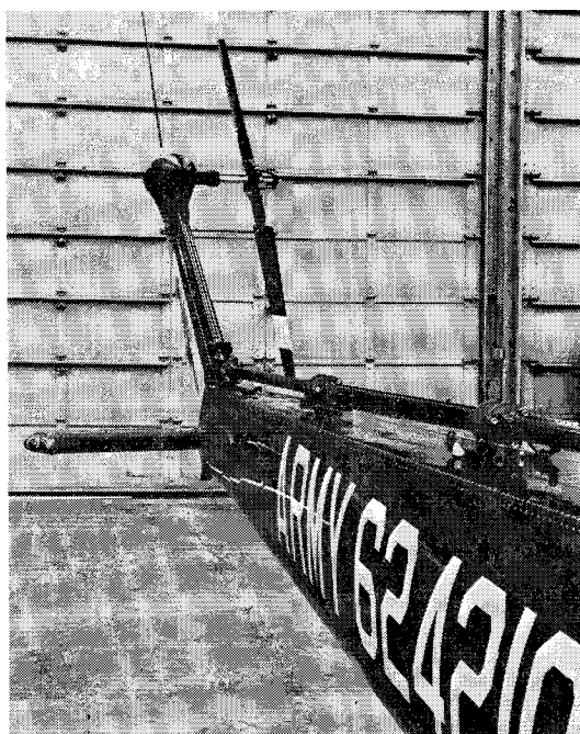
Fig. 4 Hiller OH-5A tail rotor system.
